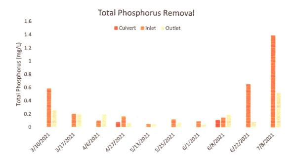
The culvert is before the water goes to the wetland. The inlet is right before it goes into the filter and the outlet is when it leaves the filter.
